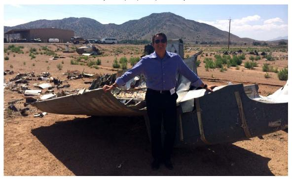
(Above) Novelist A.C. Frieden stands next to debris from a USAF B-1 bomber. This crash was blamed partly on a poorly designed fuel line that ruptured, causing an uncontrolled fire.
