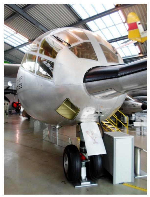
(Above) One of only two prototypes of the Dornier Do 31, the world's only VTOL (Vertical Take-Off and Landing) fixed-wing jet-powered transport aircraft, which was originally designed to carry up to a 3-ton vehicle in the cargo bay. It never entered production but remains an example of a highly innovative design.
