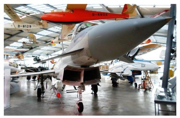
(Above, left) The Eurofighter EF-2000 DA1 (DA=Development Aircraft) on display at the museum is the first prototype of this aircraft to fly. It is one of the most modern high-powered military aircrafts and replaces the old jet fighter type F-4F Phantom and most of the Tornado fleet of the German Air Force. The Eurofighter is also in service with the air forces of three other European nations.
